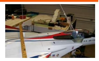
6...With the model level, lower the plumb bob until the point just touches the fuselage.
