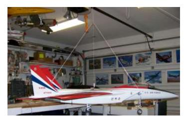
1...Set the model up on a bench or table, gear down, tank empty or battery installed and the C.G. marked on the upper part of the fuselage.
