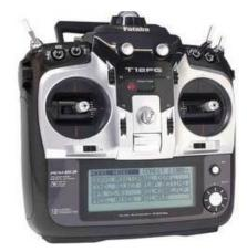
*Futaba T12FG 2.4GHz Transmitter-FASST coding-Stick Mode 1* # G3 2048 resolution # 30 model memory, or expand up to 1,882 models
